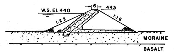
SECTION OF THE RIVERSIDE DAM (Scale 1:1000)
