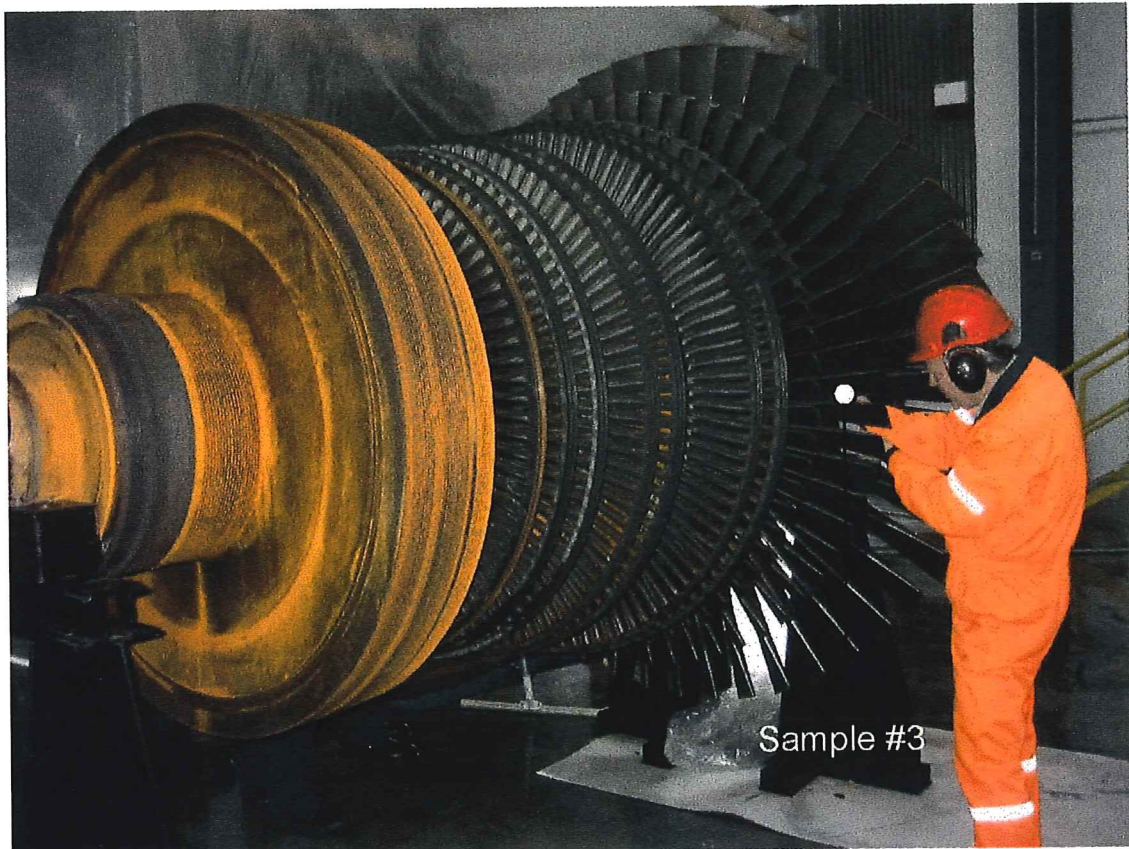
Figure 4. Turbine rotor after washing. Sample #3 was a very - very thin film from the 8 th stage.
