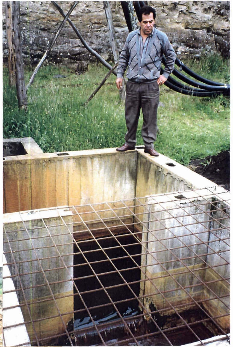
Picture 7. The water overflow from San Guillermo through the rectangular weir was used to measure the flow.
